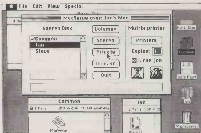
Macserve lets network users share a hard disc; two private partitions and one shared are being used here.
